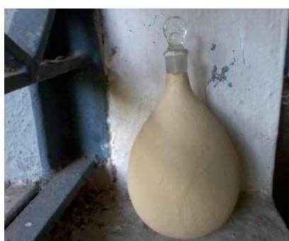
4) 150 ML GLASS FLASK WITH SINGLE LAYER OF KAPADMISTI
