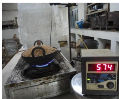
7) MAXIMUM TEMPERATURE OF KUPIPAKWA
