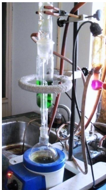
Fig-3. Methanolic extract with the help of Soxhlet apparatus.
